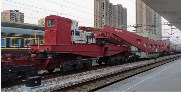
Figure 14: The freight train with transformer transport from Shaling to Shuangzhai.
